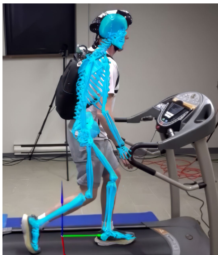
Mark and the team used a markerless motion capture system to measure how different DBS frequency settings affect gait and arm swing patterns.
